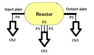
The plant consists of reactor and two pipes. The measurement points P1, P2 and P3 are for measuring the temperature, pressure and liquid level in the reactor. Points P4 and P5 measure the liquid flow speed in pipes.
